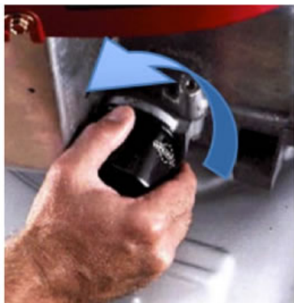
Figure 1. Replace the oil filter by twisting counterclockwise on the filter casing. Image retrieved from Briggs & Stratton (2009).
